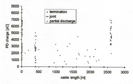
In that case, we can see that one joint got PD at about 400 m from the cable origin as well as another defect in "full cable" (electric or water tree) at about 2600 m from the cable origin.
